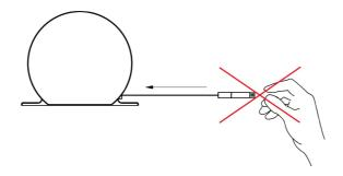
Always keep the wire aligned not to damage the equipment (maximum deviation: 3°).
